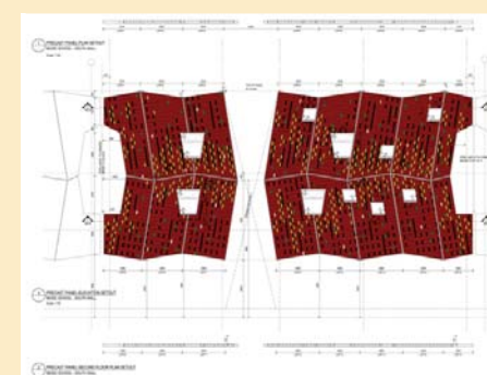
Pre-cast concrete panels with brick snaps
